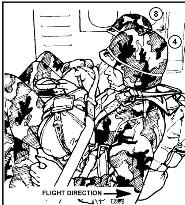
Figure 17-13. Numbers 4 and 8 with static line bight and safety belt secured.
